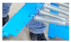
9. After you have sprung the bed, there will be 1-3 extra holes in the frame. These additional holes are there in case you need to skip another frame hole to make the bed tighter.
