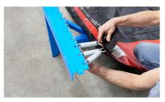
3. Hook the first and second springs into the first D-ring. The third spring should go into the second D-ring and so forth.
