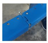
3. Match the knuckles of the rails and insert the bolt to fasten together. Secure with the nut. Make sure the nut is on the inside of the frame.
