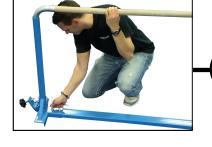
Once the bar assembly is seated all the way in the upright, finish tightening the screws in the center support.
