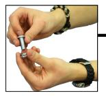
Place the screw through the lock washer and then the flat washer. Repeat for all 8 screws.
