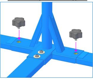
(4) Align tube holes and insert spring-knobs
